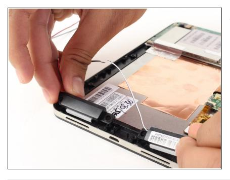
Lift the two speakers out of the device and set them aside.
