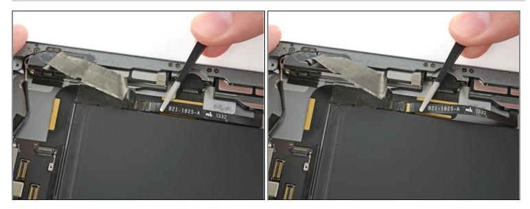
• Slide the speaker cable straight out of its ZIF connector.
