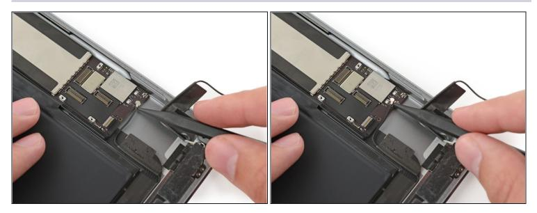
• Insert a spudger under the left antenna cable, the connector farthest from the edge of the iPad. Lift upward to disconnect the antenna cable connector.
