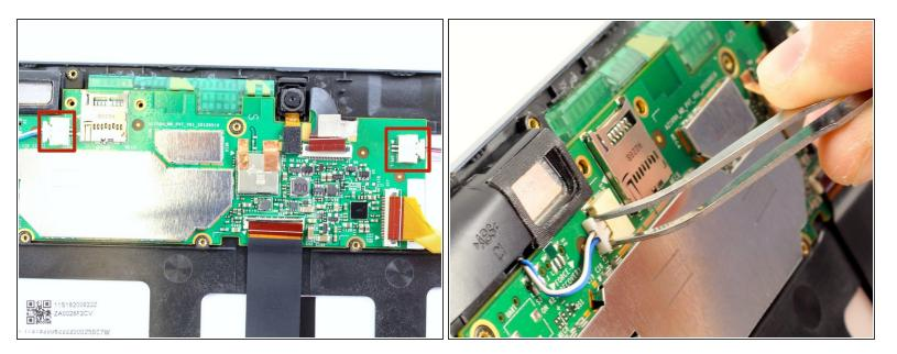
Disconnect the two speaker connectors by pinching them with tweezers and sliding them out from the system board housing.
