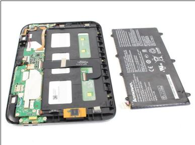
Now you can take the battery out in order to either replace it or continue disassembling the device.
