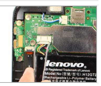
Disconnect battery power connector by pinching the connector with tweezers, and sliding it out of the housing.
