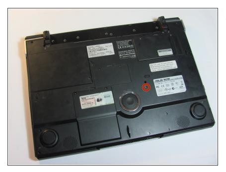
Use a Phillips head screwdriver to remove the one 3mm screw labeled
