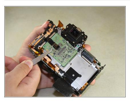
Use tweezers to remove the small metal plate and the thin strip of black tape underneath it.
