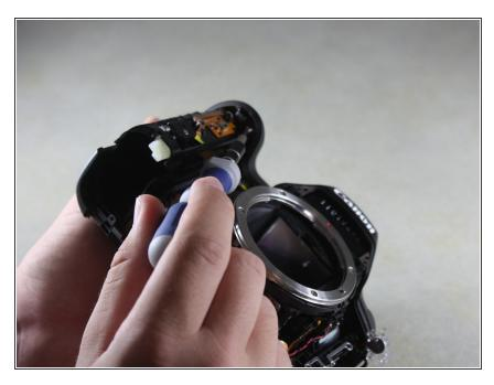
Remove the 4mm Phillips #00 screw from the inside of the top panel, below the shutter button.
