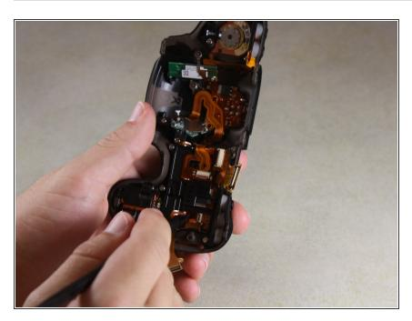
Use the pointed end of the spudger to slide out the two light brown ribbon wires.
