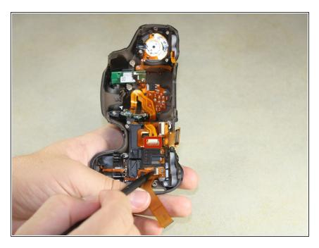
Use the pointed end of the spudger to flip up two silver ribbon wire latches on the inside of the top panel.
