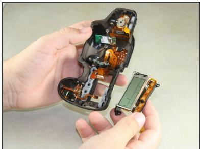
• Carefully slide the flat end of the spudger underneath the screen and lift it out.
