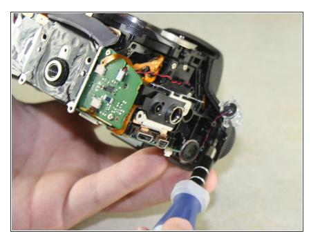
Remove the 4mm Phillips #00 screw from the inside of the top panel, below the strap hook.
