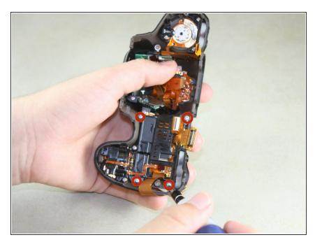
Remove four 5mm Phillips #00 screws from the inside of the top panel.
