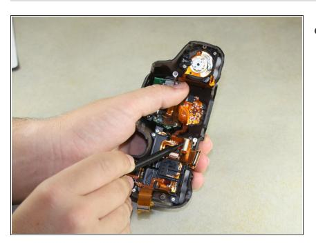
Use the pointed end of the spudger to carefully remove the third light brown ribbon wire.
