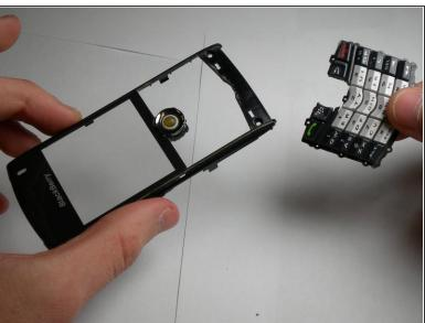
Gently remove the keyboard from front casing. It should snap out of place.
