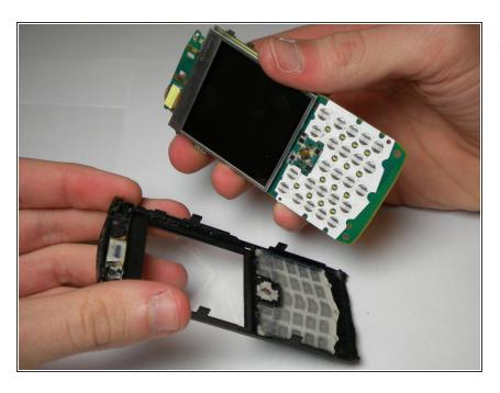
Separate the logic board from the front panel.
