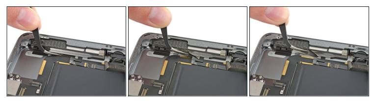
• Remove the tape holding the speaker to the rear case.
