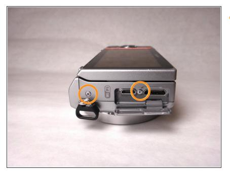
Open the HDMI port, and remove the the two (3.5 mm) Phillips screws exposed on that side.
