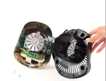
Remove the plastic bottom from the base of the blender.
