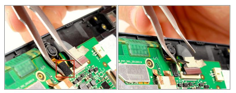
Use tweezers or your finger nail to disconnect the camera attachment by flipping up the black rectangular connector.
