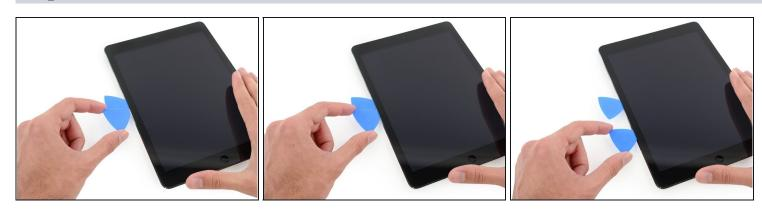
• Place a second opening pick alongside the first and slide the pick down along the edge of the iPad, releasing the adhesive as you go.
