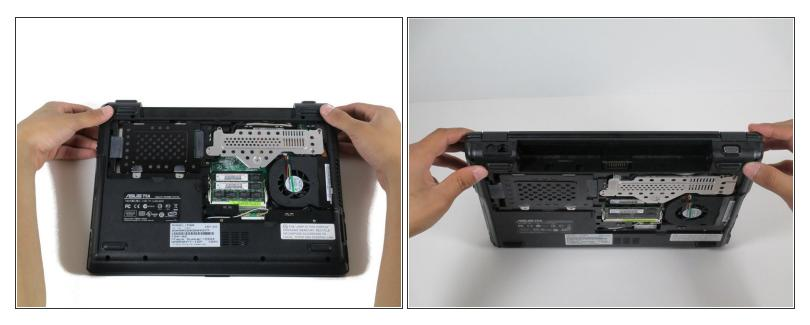
Rotate the laptop 90 degrees towards you so that you are looking at the empty battery compartment.
