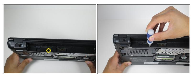
• Remove the 2.0 mm Phillips #3 screw located beneath the battery compartment.
