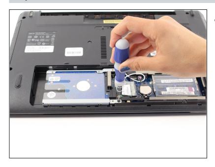
Remove the two screws using a Phillips #00 screw driver.
