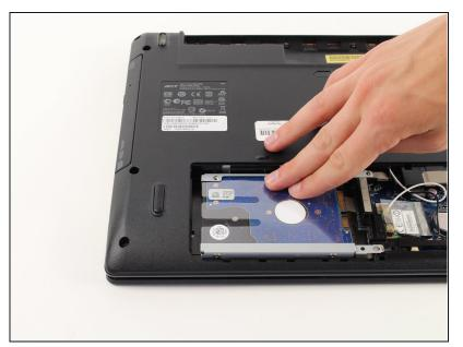
Carefully slide the hard drive in the opposite direction of where the screws are located until it dislocates.
