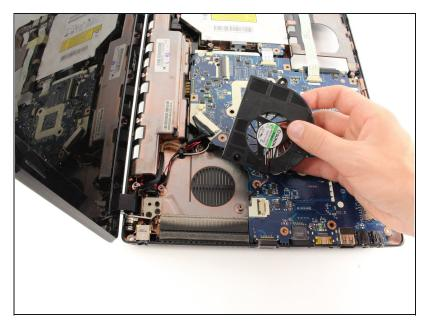
• Carefully lift the fan out of place.
