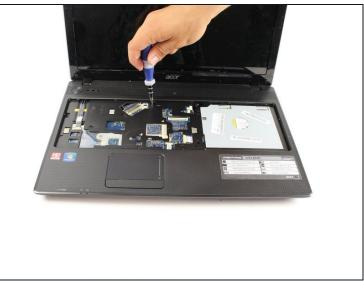
Flip the Laptop back over, and unscrew the 1/4" diameter head 7/32" length screws indicated in the picture.
