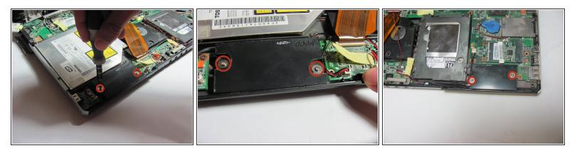
Remove the 2.4 mm, wide Phillips screws per speaker holding in the two speakers at the lower end of the device.
