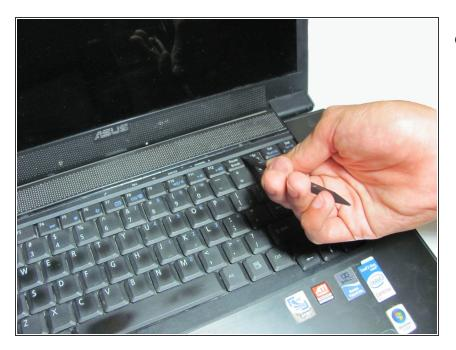
• Remove the panel above the keyboard with a plastic spudger.
