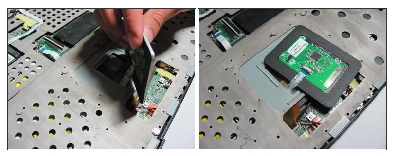
• The touchpad should be loosely attached to the rest of the laptop by a ribbon cable.
