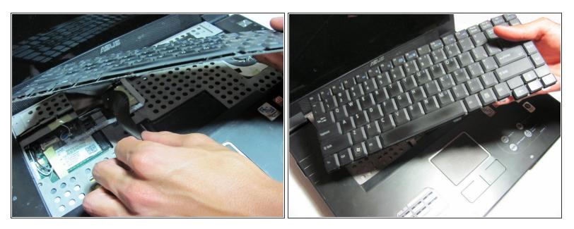
• Detach the ribbon cable from the keyboard by pulling the end of the ribbon cable that is attached inside of the laptop.
