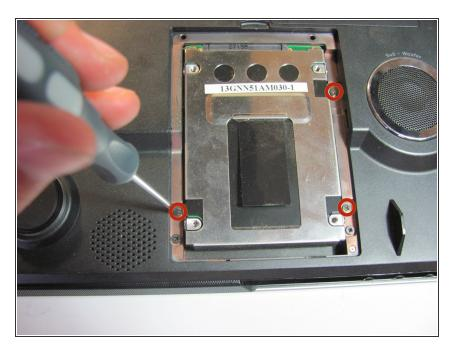
Remove the 3 4 mm Phillips upper screws holding the hard drive down.
