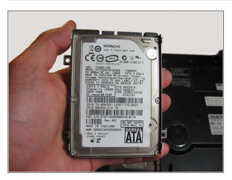
Lift the hard drive upwards to remove it from the laptop.
