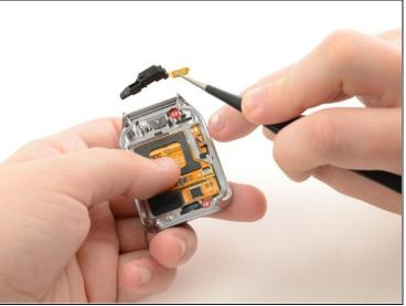
• Use <u>tweezers</u> to grab the orange connector that is attached to side the home button assembly and lift to remove it from its adhesive.
