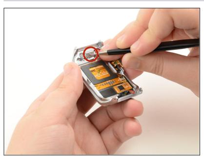
Use either the tweezers or the spudger to push the button peg out through the hole.
