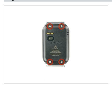
Remove the four 4.0 mm screws on the back of the Gear using a T5 Torx Screwdriver.
