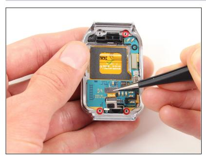
Use tweezers to carefully lift the camera from its slot out of the case.
