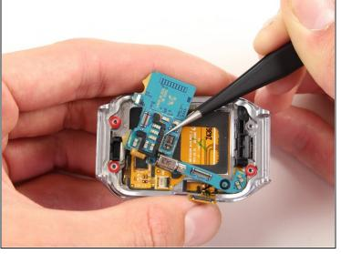
• Once the safety belt is removed, use tweezers to take the motherboard out of the Gear 2.
