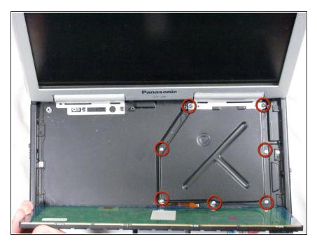
Remove screws shown from cover plate
