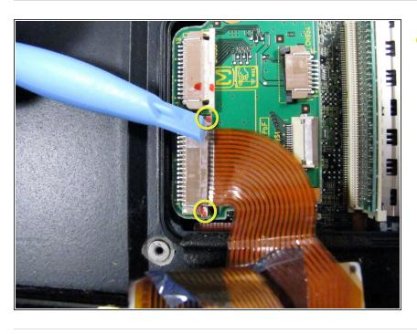
Remove both ribbon cable by pulling
