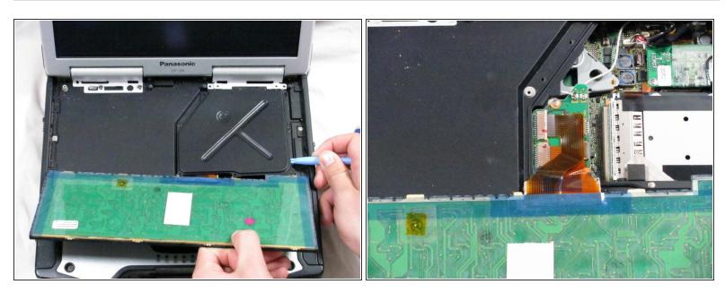
Pull cover plate out of place revealing the ribbon cable connections to the motherboard
