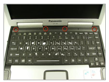
Remove the four screws above the keyboard using a Phillips #0 screwdriver.
