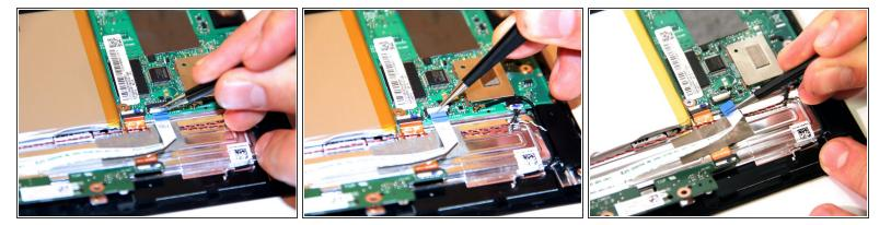
Lift up the power button cable retention clip on the motherboard and pull the cable out.
