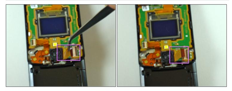
• Firmly grab the flexible circuit with <u>tweezers</u> to detach (or use your fingers if you can manage a firm grip).
