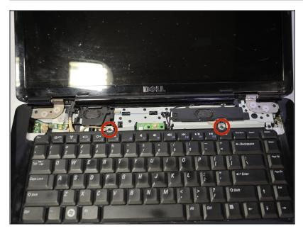
Remove the two screws (5mm Phillips #1) at the top of the keyboard.
