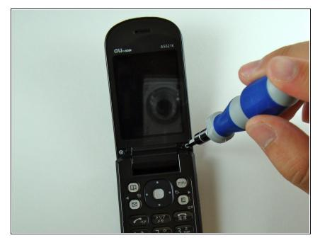
• Remove the screws using a Y0 screwdriver.
