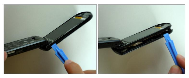
• Use the iPod pry tool to loosen the faceplate from the phone.
