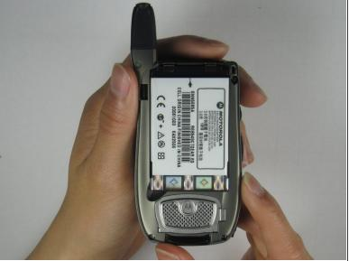
Slide the back cover towards the antenna while lifting the cover away from the phone.
