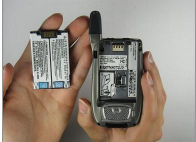
• Lift the battery out of the phone while pushing it towards the antenna.
