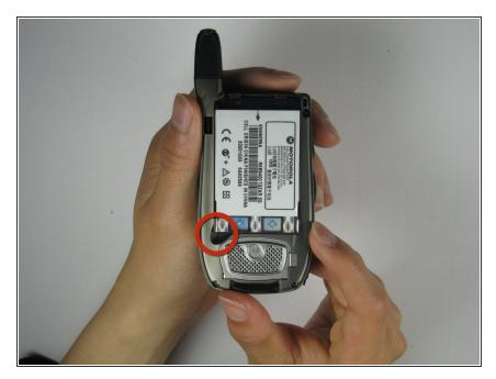
Place your thumb on the indicated corner while stabilizing the phone and the upper portion of the battery with your forefinger.
