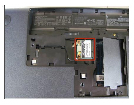
Locate the wireless module next to the RAM slots.
