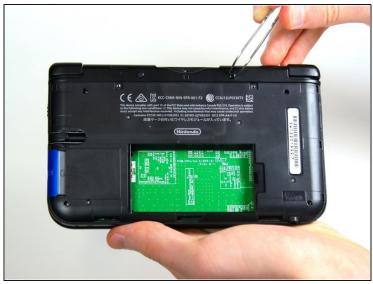
• Using <u>tweezers</u> pull out the rubber bumpers that are located at the top of the device on either side of the game cartridge compartment.
