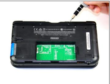
• Remove the six 6.2 mm screws using a Phillips #00 screwdriver
