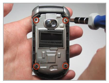
• Using the T6 Torx Screwdriver remove all 4 small screws.
