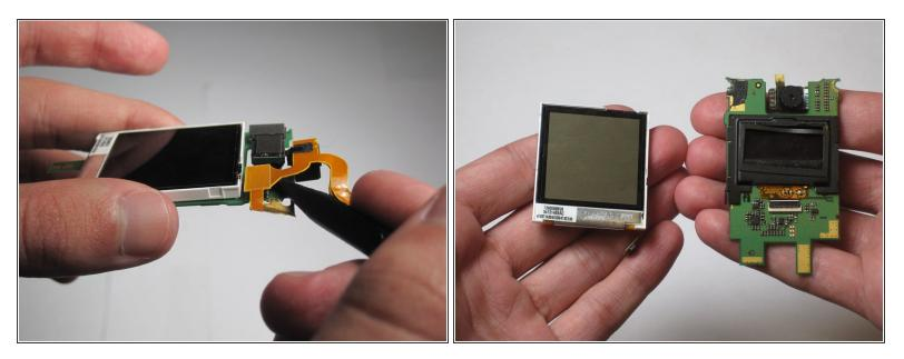
• Using spudger remove the LCD screen from the green logic board.
