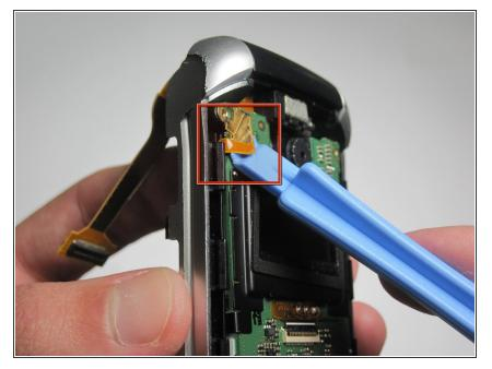
Using the iPod Opening Tool remove the yellow flex cable from the green logic board.
