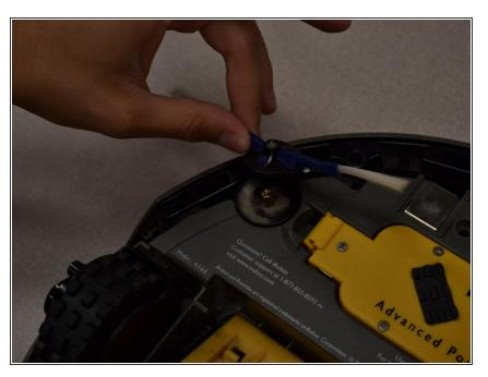
• Gently pull the spinning brush upwards to remove it.
