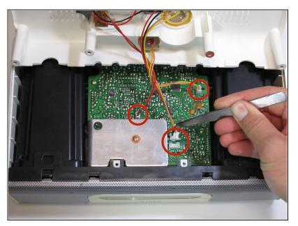
Use tweezers to unplug the three wires connected to the circuit board. If the wires are tight pliers might work better.
