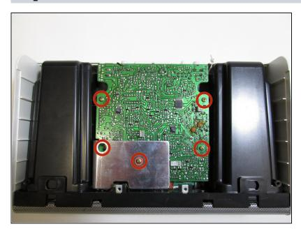
• Remove the five 5/16 inch screws from the circuit board.
