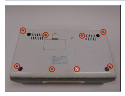
Remove the eight 5/16 inch screws with a #2 Phillips screwdriver.
