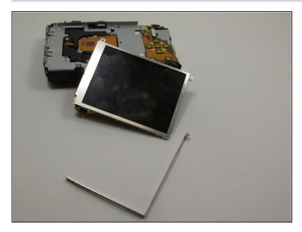
Remove the indicated "L" shaped bracket from around the top and right side of the LCD screen.
