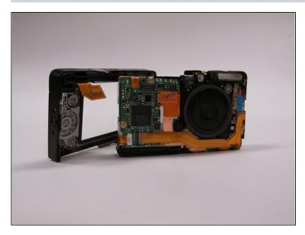
Carefully pull the case apart at the seam. The case will detach from the camera in two pieces.
