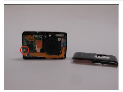
Remove the screw on the far lefthand side of the front of the camera using a Phillips #00 screwdriver.
