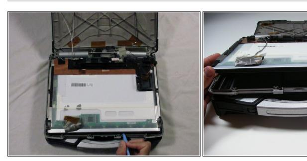
Using a plastic opening tool, lift the screen as shown from the case and pull free.
