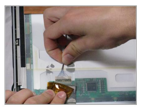
Pull the wiring away from the connection to release it.
