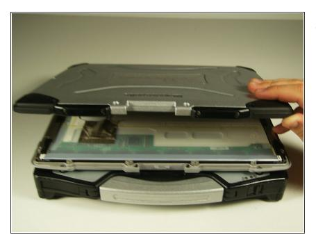
Pull the top halve of the casing up revealing the inside of the screen
