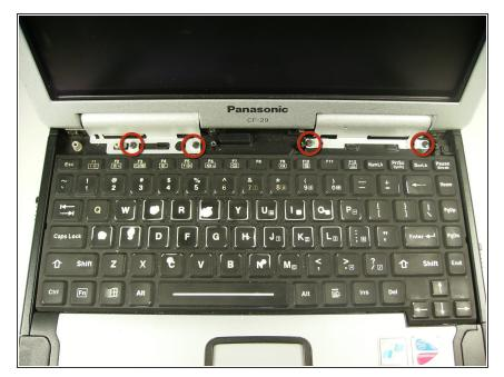
Remove the four hinge screws to allow the hinges to rotate up and move.
