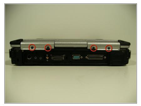
Remove the four hinge screws from the back of the computer.
