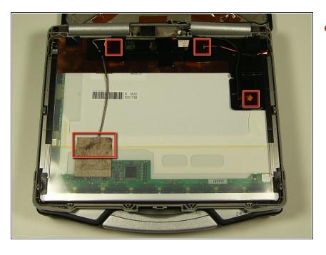
There are 4 wires that need to be unplugged to remove the screen.
