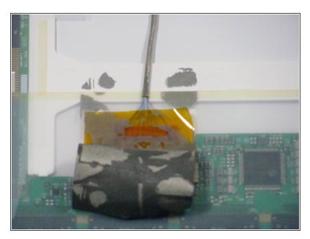
For the first wire, peel back the silver cover tape to reveal the connection.
