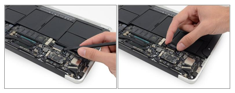
In this step you will disconnect the battery to help avoid shorting out any components during service.
