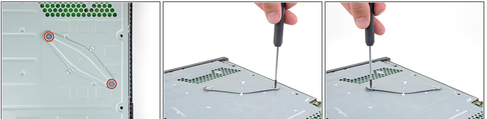
**i** This step shows you how to properly unscrew the pressure plate.
