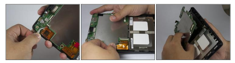
After all ribbon cables are disconnected, move them out of the way, and the motherboard should fall out easily.
