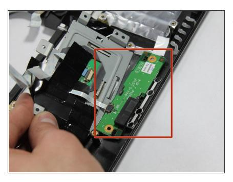
Slide green circuit board to right and lift track pad free from laptop.
