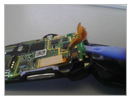
• Using a small plastic opening tool, remove the motherboard.
