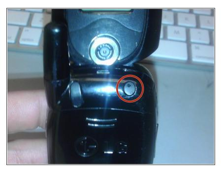
Using a spudger or plastic opening tool, pry off the screw cover near the phone's antenna.
