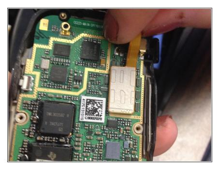
• Carefully disconnect the gold ribbon cable from the upper right corner of the motherboard.
