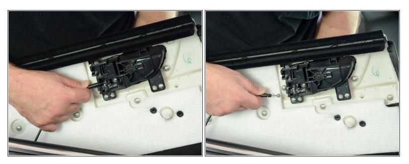
Repeat the same procedure above with the black cable. First disconnect the black sleeve, then the ball, and finally move the entire cable away from the door panel.
