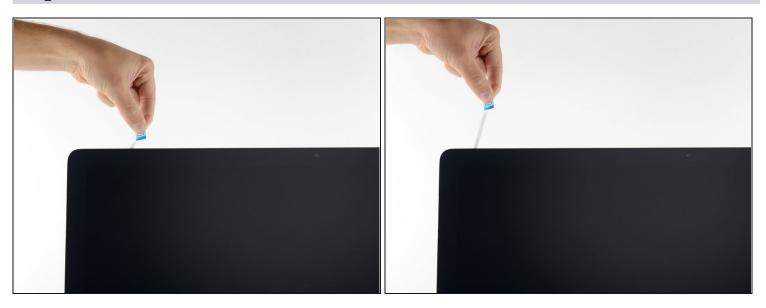
• Remove the other side of the protective film from the top left strip.
