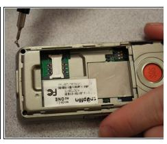
• Remove the four 3.1mm screws in the corners with a Phillips #00 screwdriver.
