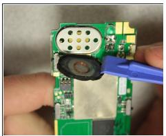
• With the plastic opening tools, pry off the speaker from the circuit board.
