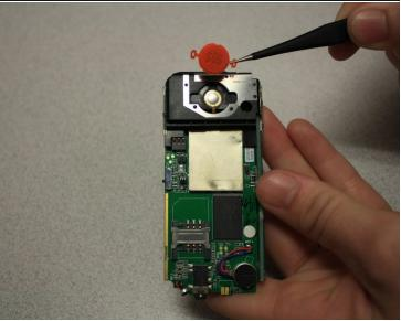
Remove SOS button from circuit board with tweezers.
