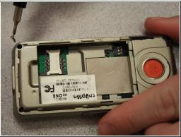
Remove the four 3.1mm screws in the corners with a Phillips #00 screwdriver.
