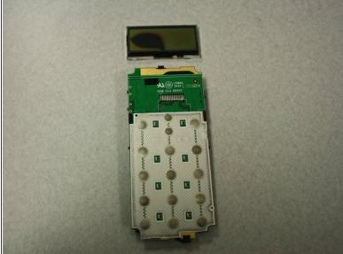
Once you heat the solder connection, lightly tug the ribbon cable free. The LCD screen will be completely removed from the device. To reassemble your device with a new LCD screen, follow these instructions in reverse order.
