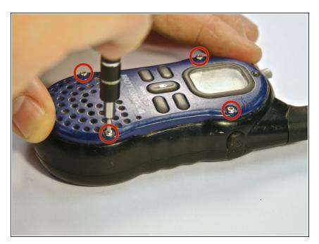
Remove the four 3 millimeter T6
