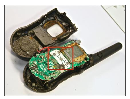
The button contacts can be seen in the red box of the picture.
