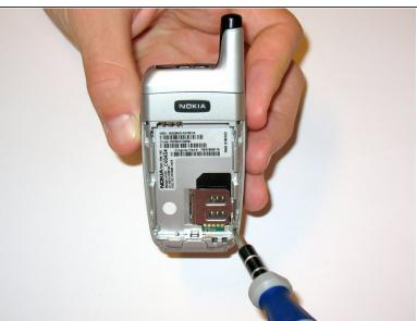
Using a .208 head <u>T-6 Screwdriver</u> remove the two screws at the bottom of the battery cavity.
