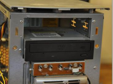
Remove the optical drive completely from its port.
