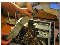
• Pull the ribbon cable out of the back of the optical drive.
