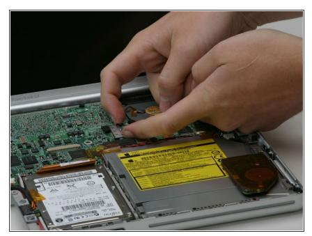
Remove the two pieces of orange tape covering the display data cable and disconnect the cable from the logic board.
