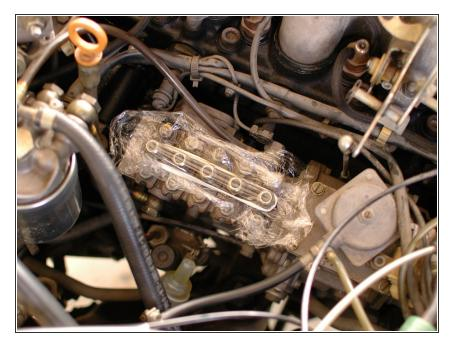
• While your hard lines are off, cover the hard line fittings on the pump as well as at each injector to prevent contamination from entering. The injector nozzles have very small openings that can be easily clogged.
