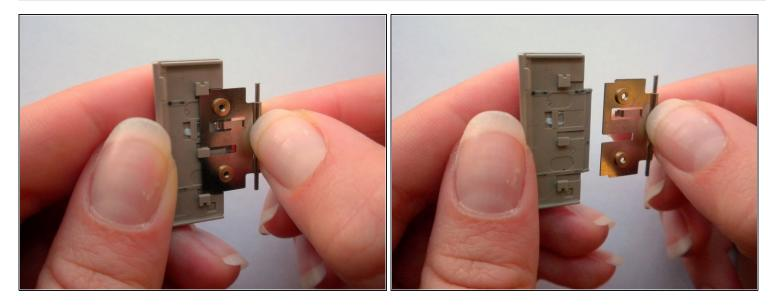
• Slide the metal piece off of the battery cover.
