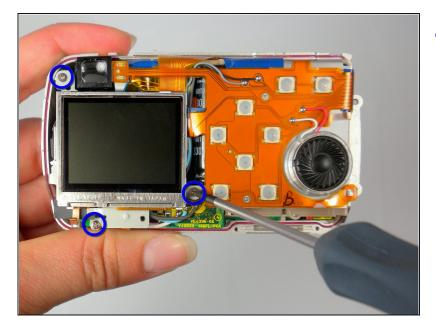
Locate the 3 internal screws holding on the front of the case. Remove them with a #00 Phillips screwdriver.
