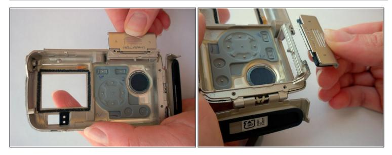
• Open the battery cover and lift it up and off of back camera case.
