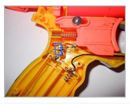
Use a hot soldering iron to melt the solder of the two wires at the rear of the switch. Take note that the red wire leads from the top of the switch.
