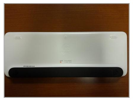
Turn the keyboard over and slide the battery cover in the direction of the arrows slightly, and then lift the cover away.
