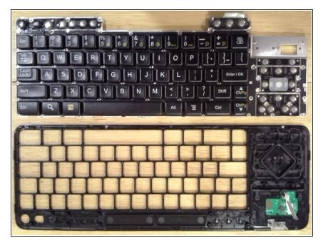
Should you go further and remove the 12 screws and 35 plastic rivets, you can see this.
