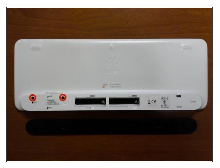
Remove the batteries and the two screws shown.
