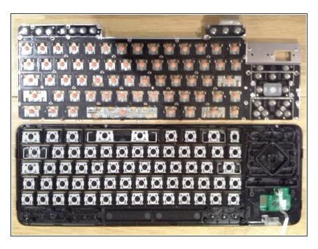
The keys can be popped out easily enough by pushing from the back side. This exposes the key matrix.
