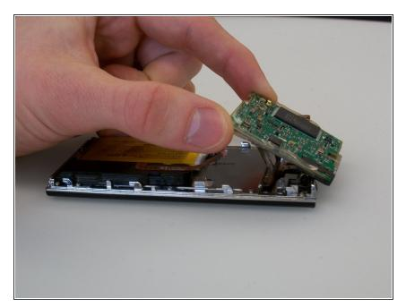
Disconnect the battery connector, and then lift the circuit board up.
