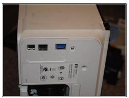
T10 bit; time to start unscrewing.
