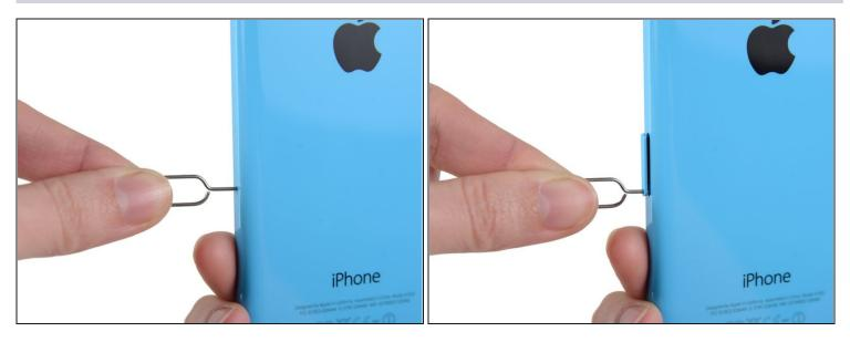
(i) Shut your phone down completely before removing the SIM card and tray.
