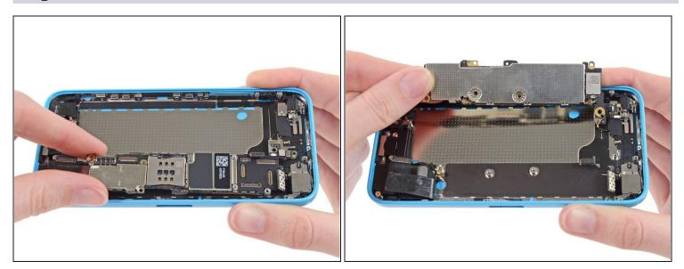
• Flip the logic board up toward the volume control buttons to expose the antenna connector.
