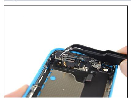
• Remove the vibrator motor.
