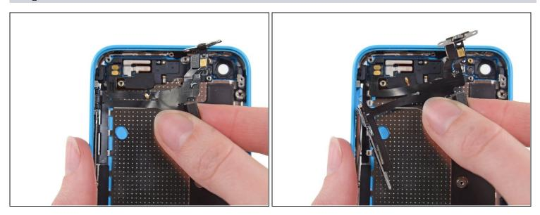
• Peel the upper assembly cable up from right to left to separate the adhesive holding it to the case.
