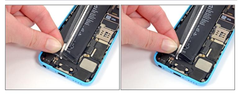
• Cut the black battery adhesive tab between the two white adhesive strips, separating them.
