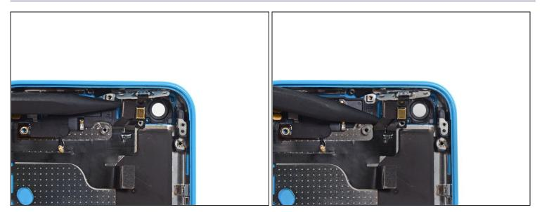
• Run a spudger gently under the flash assembly cable to separate it from the phone.
