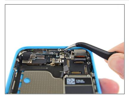
• Use tweezers to remove the logic board grounding clip.
