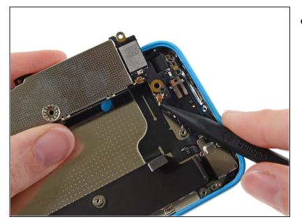
• Disconnect the antenna connector from the back of the logic board.
