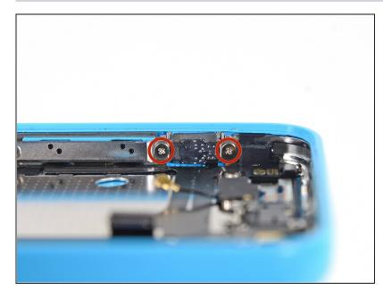
• Remove the two 1.6 mm Phillips #000 screws from the mute/silent switch bracket.
