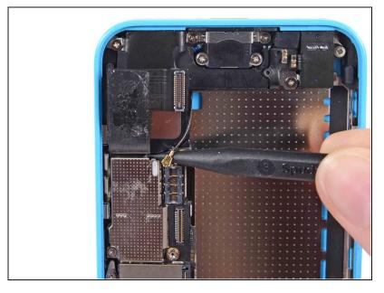
• Disconnect the lower antenna connector from the base of the logic board.
