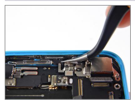
• A small piece of tape may obscure the logic board grounding clip. If so, use a pair of tweezers to remove the tape.
