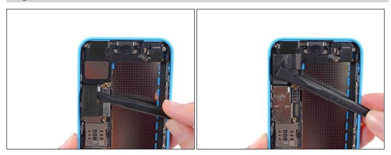
• Flip the Lightning connector cable up out of the way of the logic board.
