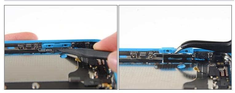
• Use the tip of a spudger to fold the volume rocker bracket down from the side wall. Remove the volume rocker.
